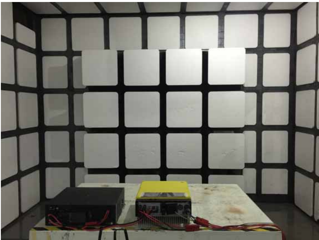
Back View of R/S Test
