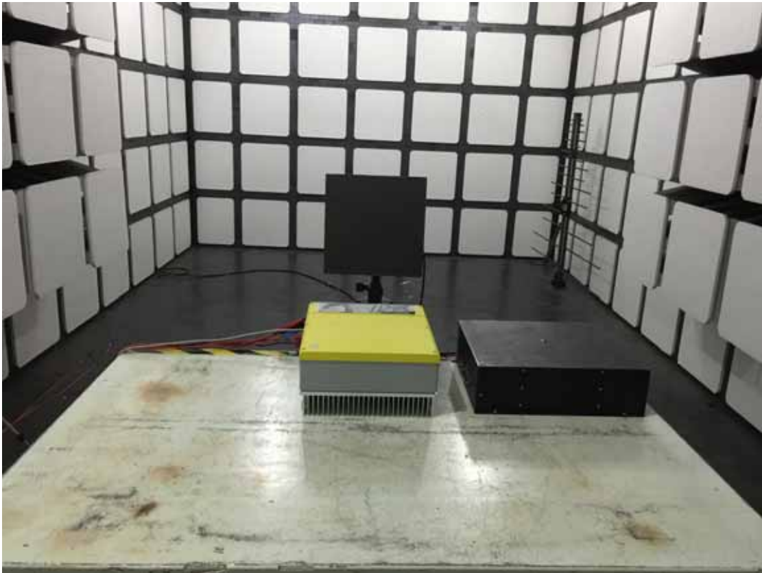
Front View of R/S Test (Above 1GHz)
