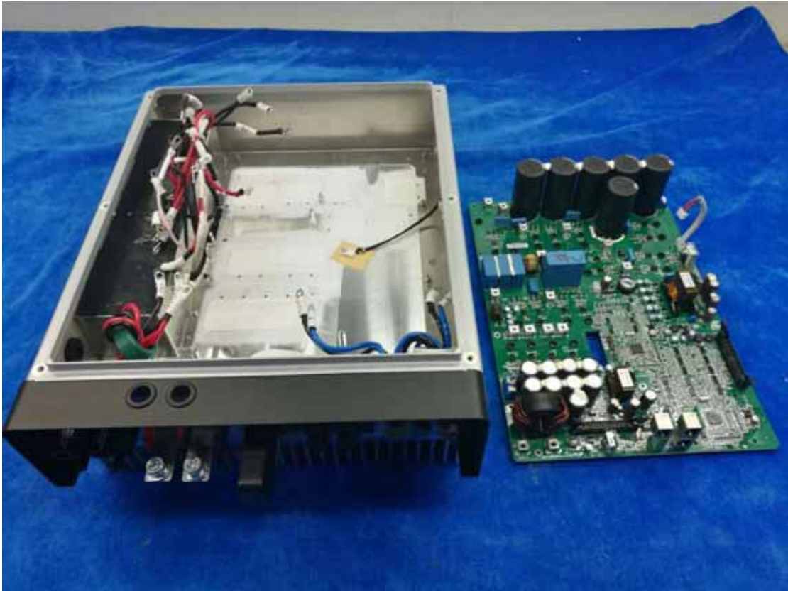
Figure 17 PCB Board Removed
