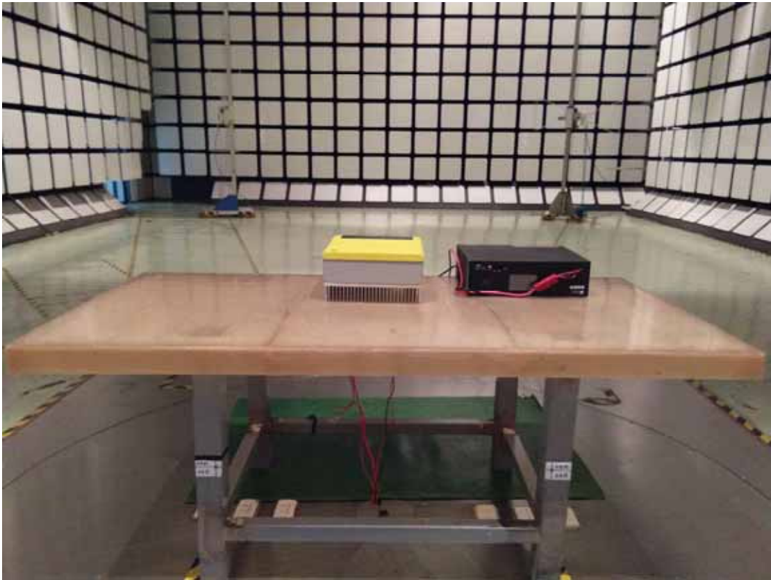
Front View of Radiated Disturbance Measurement
