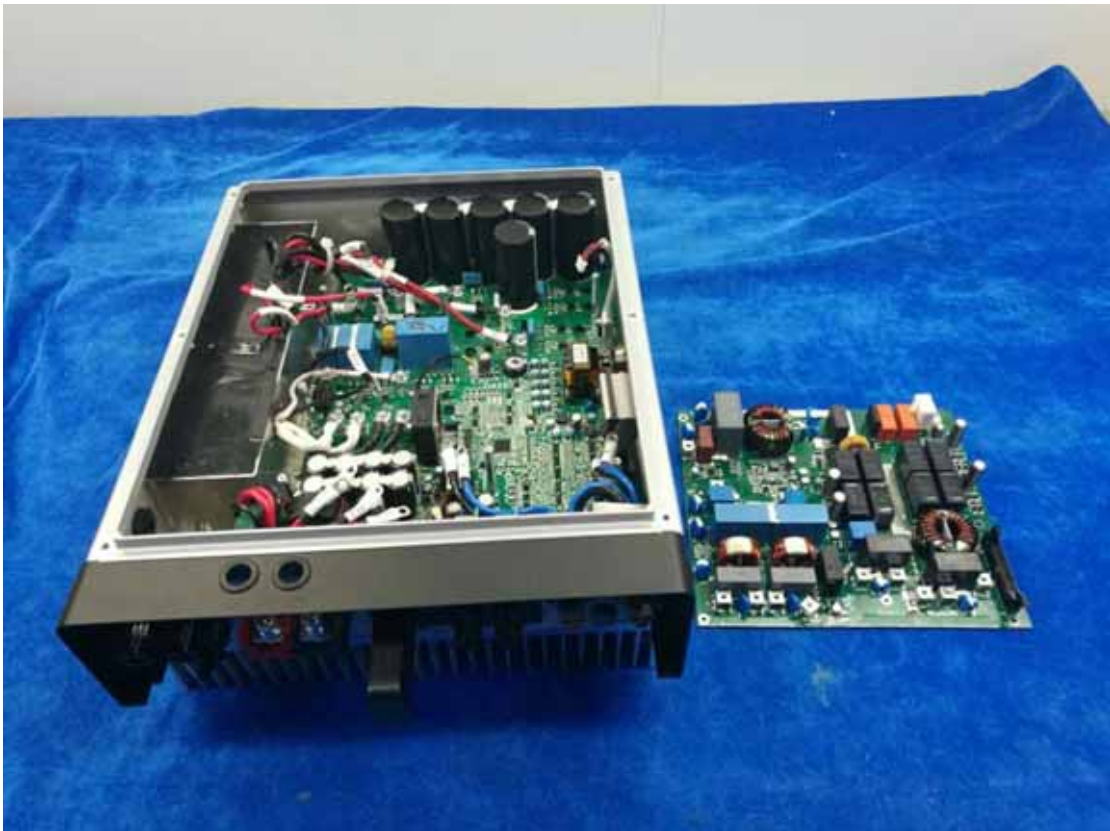
Figure 14 PCB Board Removed
