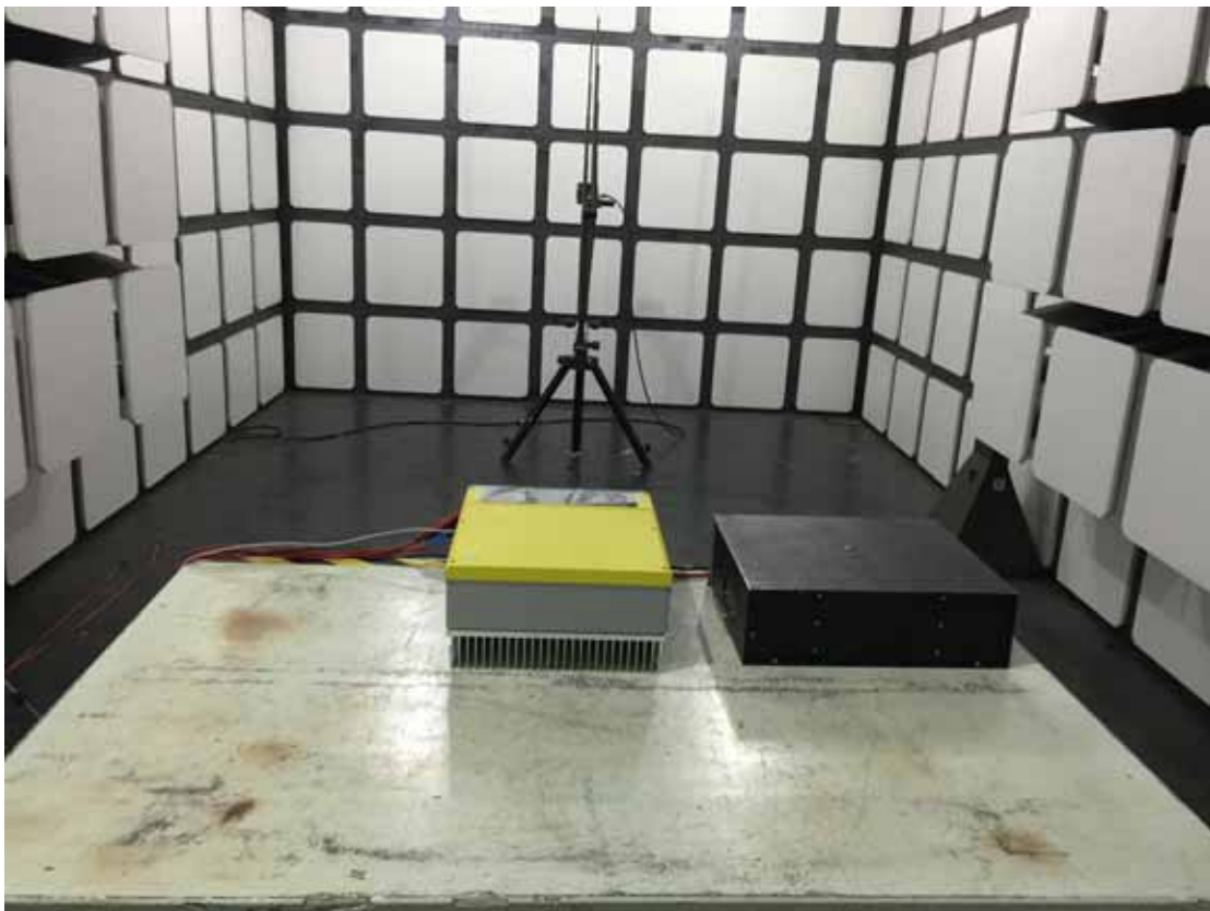
Front View of R/S Test (80MHz~1GHz)
